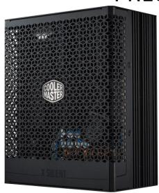
Introducing the X Silent Edge Platinum 230V, the industry's first PSU to achieve 1100W. The Edge features totally silent and dustless performance, innovative heat pipe technology, advanced heat dissipation, 80 Plus Platinum efficiency, an active bridge rectifier, and a digital monitor powered by Cooler Master's MasterCTRL software. With these features, the Edge provides precise and silent power.
